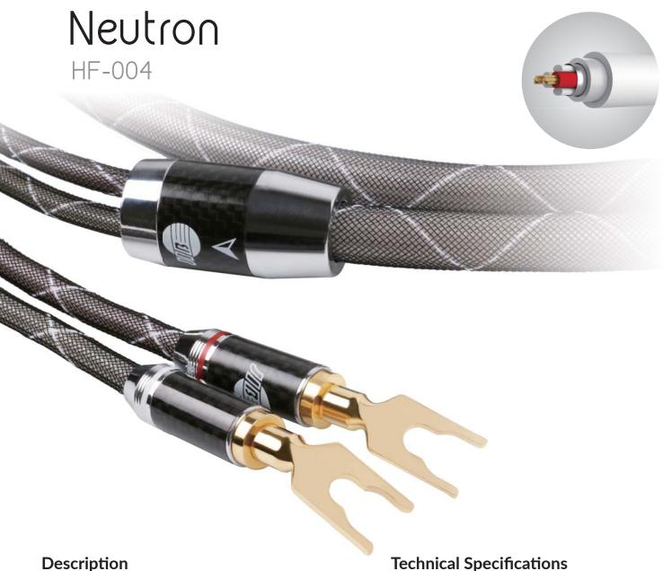
The loudspeaker cable HF-004 has twin symmetrically constructed multi-strand wire conductors sheathed in cotton braiding, each having a 2.0702 mm<sup>2</sup> cross-section, made from high-quality copper using OCC® (Ohno Continuous Casting) technology and having a material purity of 99.9999%. The contact surfaces of the interchangeable spade or banana plugs (both included) are 24k gold plated for absolute corrosion resistance and loss-free signal transmission.
